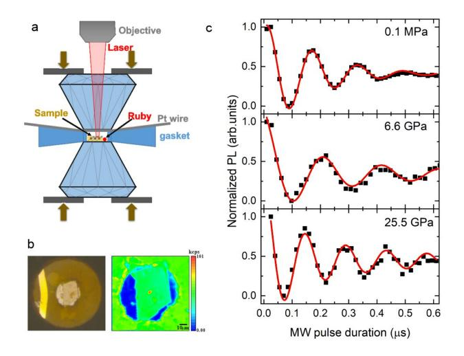
The optical and spin properties of silicon carbide divacancy defects under high pressure were studied by using diamond anvil cell. Credit: Liu Lin
