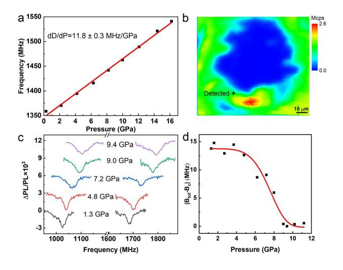
Detection of pressure-induced magnetic phase transition of a Nd2Fe14B magnet using PL6 defects. Credit: LIU Lin
