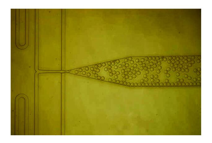
A microfluidic device was designed to combine protein solution with nanoparticles and then form thousands of tiny, identical droplets. Inside each of these droplets, the proteins interact with the nanoparticles, which help them to form protein crystals. Credit: Massachusetts Institute of Technology
