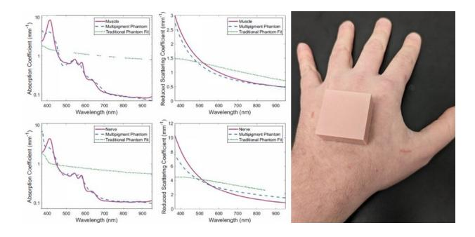
Multipigment phantoms match the optical properties of their target tissue more accurately than traditional phantoms across the entire near infrared—visible light spectrum. Right: Photo of a phantom made to match to the optical reflectance of a hand. Credit: Alec B. Walter (Vanderbilt University).
