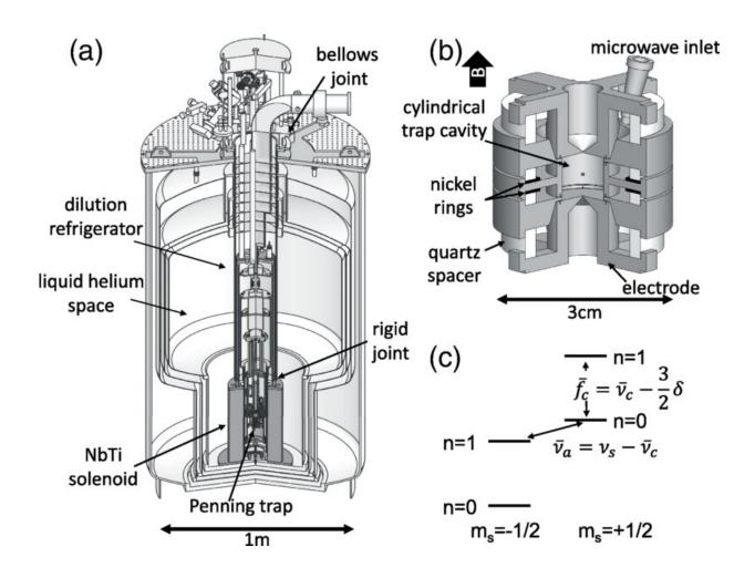
(a) Cryogenic system supports a 50 mK electron trap upon a 4.2 K solenoid to provide a very stable *B*. (b) Silver electrodes of a cylindrical Penning trap.
