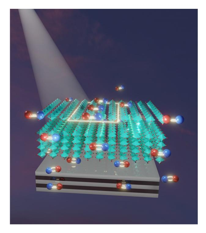
This illustration from the Guo Lab shows the interaction between a perovskite material (cyan) and a substrate of metal-dielectric material. The red and blue pairings are electron-hole pairs. Mirror images reflected from the substrate reduce the ability of excited electrons in the perovskite to recombine with their atomic cores, increasing the efficiency of the perovskite to harvest solar light.
