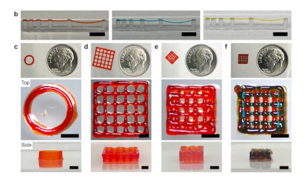
Structures printed using the peptide-based 3D-printing ink developed by Rice's Hartgerink lab. A dime is included for scale. Credit: Hartgerink lab/Rice University
