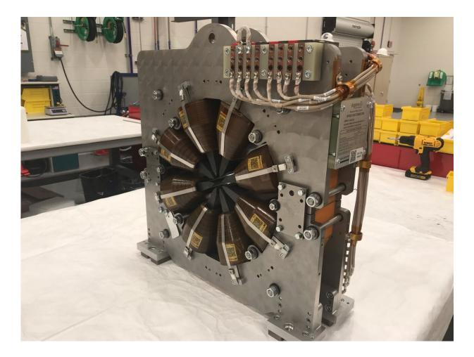
One of the eight-pole fast-corrector magnets that Brookhaven engineers designed and built for the APS upgrade project. It was the 1,000th magnet to arrive at Argonne for use in the APS Upgrade. Credit: Nicholas Bechtold
