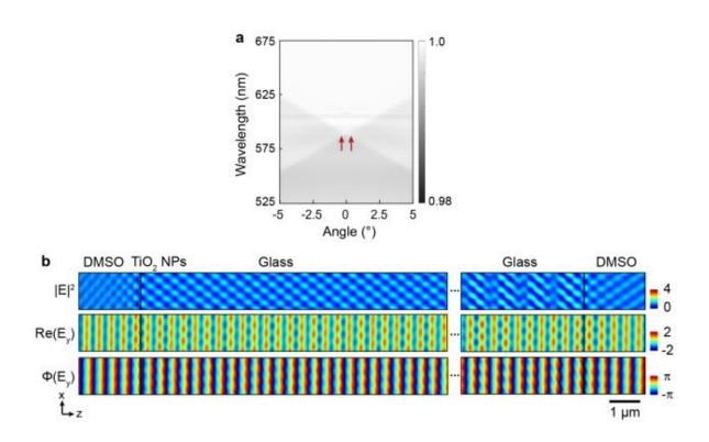
Non-plasmonic materials show weak phase modulation. (a) Simulated transmission wavelength vs. angle map shows weak photonic bands. (b) Simulated electric field distributions at 586 nm with an incident angle ~0.5°. The incident light is polarized along the y direction. Credit: *Nature Nanotechnology* (2023). DOI: 10.1038/s41565-023-01320-7
