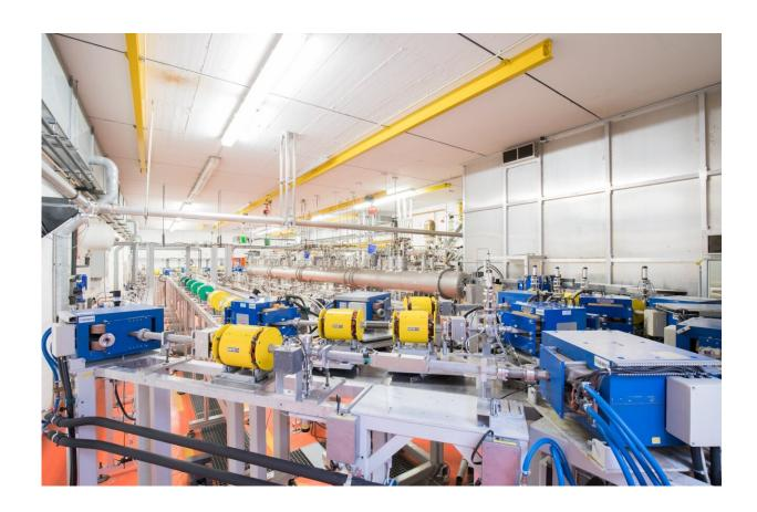
Picture of the superconducting Darmstadt linear electron accelerator (S-DALINAC) which was operated in multi-turn energy recovery mode. Credit: J.-C. Hartung Credit: Schliessmann et al.
