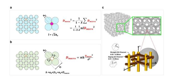
The different size ratios between multi-scale pores based on the generalized Murray's Law. (a) The size ratio between mesopore and micropore. (b) The size ratio between macropore and mesopore and (c) The hierarchically porous structural illustration of OMMM–ZSM-5 zeolites. Credit: Science China Press
