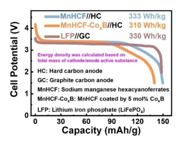
The sodium manganese hexacyanoferrate full-cell configurations show comparable energy density to that of the well-known LiFePO4 full cells. Credit: *Angewandte Chemie International Edition* (2023). DOI: 10.1002/anie.202217761
