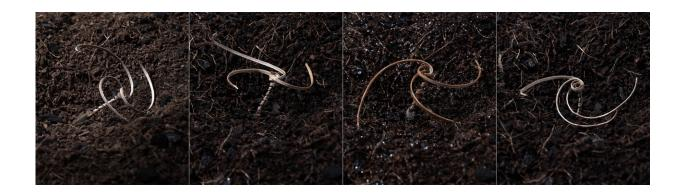
This time-lapse shows an E-seed carrier drilling into the ground after exposure to moisture. Credit: Carnegie Mellon University
