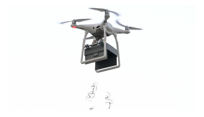
E-seeds are dropped from a drone during a field test of the engineered seed carriers. Credit: Carnegie Mellon University
