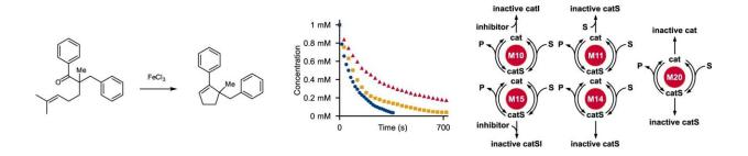
Additional case study with experimental kinetic data. Includes the reaction under study, the experimental kinetic data used as input for the AI-model and its output. Symbols correspond to substrate concentration. Red triangles: lowest catalyst loading; yellow squares: medium catalyst loading; blue circles: largest catalyst loading. Credit: *Nature* (2023). DOI: 10.1038/s41586-022-05639-4
