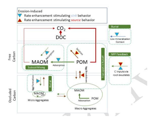
Transport in runoff: detachment and transport can shift OC from a protected state in aggregates to an available state where it mineralizes more rapidly.Burial: the deposition of eroded OC moves OC into a low-mineralization context and can also enhance protection via aggregation. Subsoil mixing: at sites of erosion
