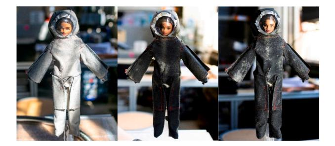
1/6-scale astronaut after dust application (left); after dust application and treatment in a vacuum (center); after dust application, treatment in a vacuum, and spot treatment with a handheld liquid cryogen spray (right). Credit: WSU
