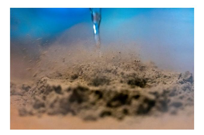
Cryoclastic flow caused by liquid nitrogen poured on lunar dust simulant. Credit: WSU
