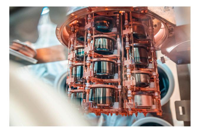
The Majorana Demonstrator's germanium crystals are suspended in a glovebox in a cleanroom on SURF's 4850 Level. Credit: Nick Hubbard
