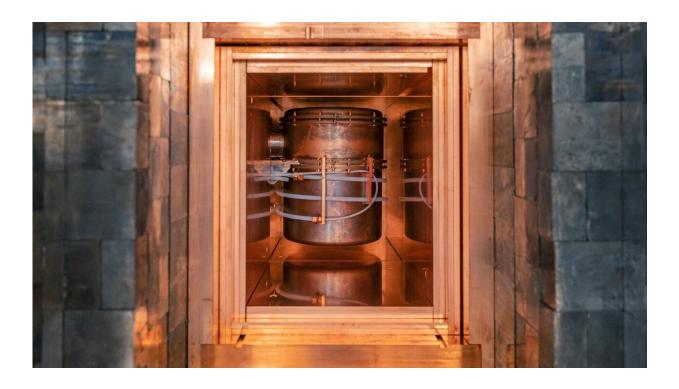
The Majorana Demonstrator's inner detector is pictured within the experiment's massive copper and lead shield. Credit: Nick Hubbard
