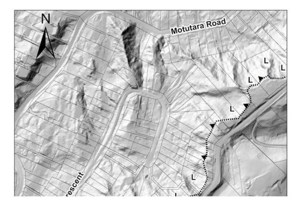
This digital elevation model shows former landslides, roads and properties in Muriwai. Credit: Martin Brook
