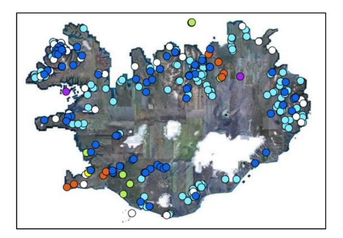
Map of power plants in Iceland. Orange dots represent geothermal power plants, dark blue dots represent hydroelectric power plants, bright green dots represent wind turbine power plants, yellow dots represent solar power plants, purple dots represent petroleum-based power plants, pale blue dots represent home power plants, white dots represent backup power plants. Credit: *Foods* (2022). DOI:
