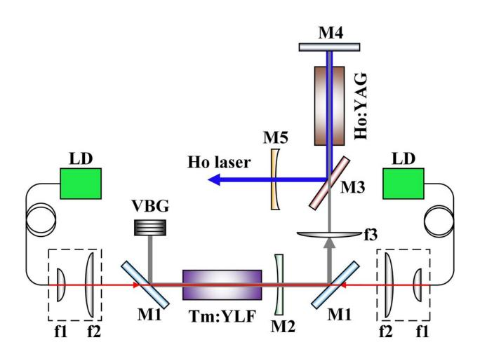
Experimental setup of the Ho:YAG laser pumped by Tm:YLF laser. Credit: *Scientific Reports* (2023). DOI: 10.1038/s41598-023-27970-0
