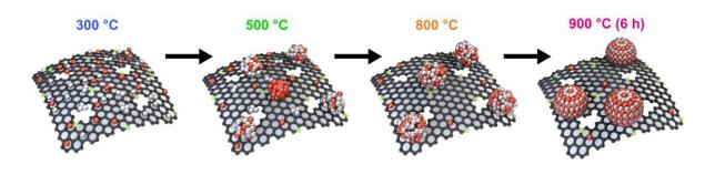
Schematic illustration of the growth process of the Co-Pt alloy nanocatalyst. Simple heat treatment at 900 °C could produce atomically ordered Co-Pt nanoparticles on a carbon support. Credit: Institute for Basic Science
