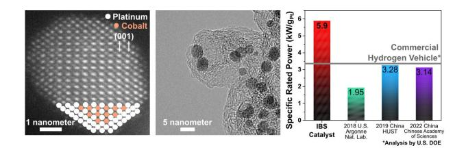
Microscopic (STEM and TEM) images of the developed catalyst and its PEMFC power performance. Compared to the state-of-the-art fuel cell catalysts, the catalyst developed by the CNR-IBS team showed almost twice the power performance per platinum use. Credit: Institute for Basic Science
