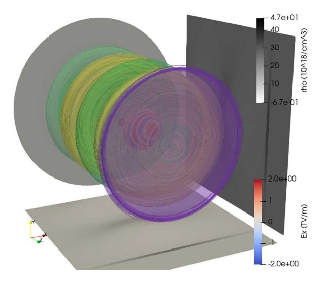
End view of a 3D simulation of the wake behind the electron beam (purple) and how a light pulse (blue and red stripe) might surf behind it. Credit: Ryan Sandberg, High Field Science Group
