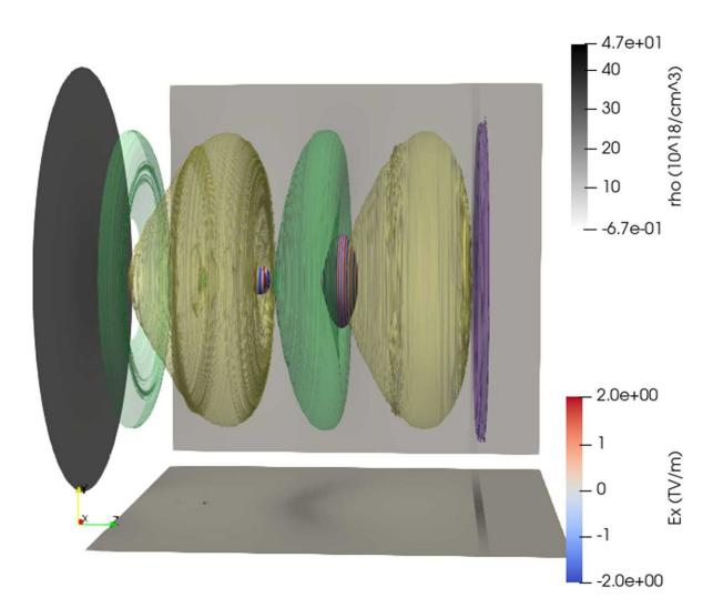
A 3D simulation of the wake behind the electron beam (purple) and how a light pulse (blue and red stripe) might surf behind it. The plasma wake is shown in
