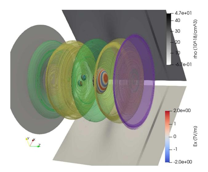
Side view of a 3D simulation of the wake behind the electron beam (purple) and how a light pulse (blue and red stripe) might surf behind it. Credit: Ryan Sandberg, High Field Science Group
