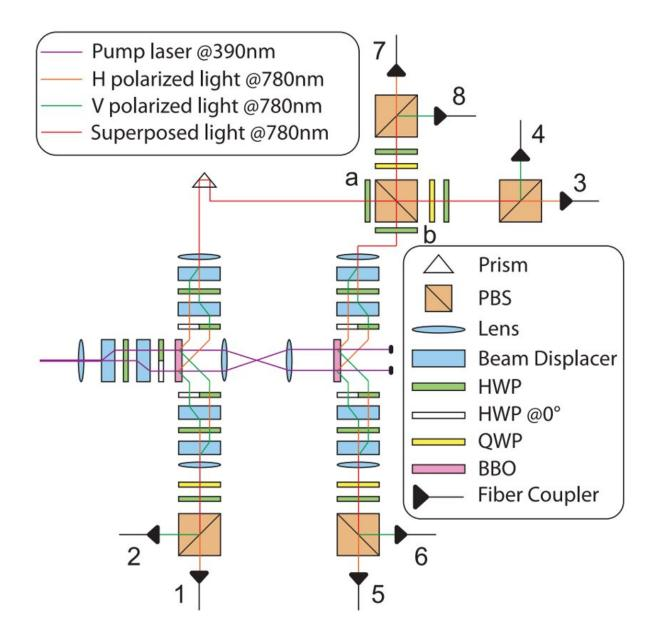
Schematic of experimental setup for generating four-photon entanglement, with the detectors labeled by order. Credit: Yang et al
