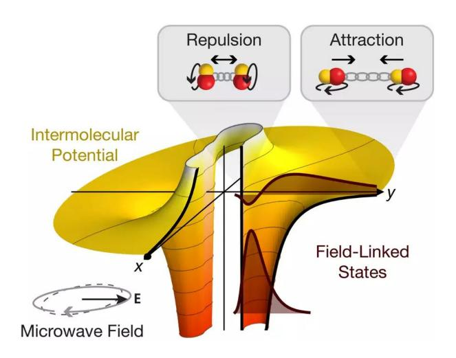
Colliding dipolar molecules experience both attractive and repulsive interactions in a rotating microwave field. With a suitable elliptical deformation of the field, so-called field-linked states are created. Credit: Andreas Schindewolf, MPQ
