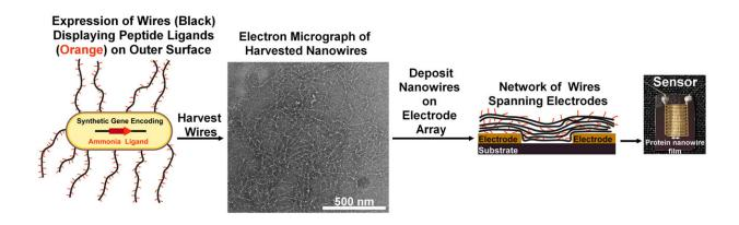
Nanowires, with their chemical-sniffing capabilities, are harvested and built into a sensor. Credit: Lekbach et al., 10.1016/j.bios.2023.115147
