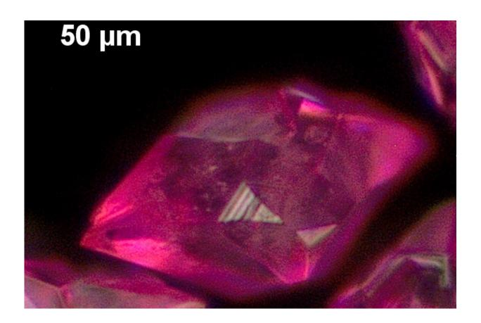
${\rm LiFe_{1-x}Co_x}$  Borophosphates (here as tiny crystals with lenghts of some 50 micrometers) could be used as inexpensive catalysts for the production of green hydrogen. Now a team at BESSY II has investigated what happens at the catalytically active molecular centers. Credit: P. Menezes / HZB /TU Berlin
