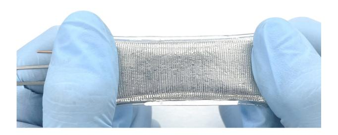
An international team of researchers has developed a technique that uses liquid metal to create an elastic material that is impervious to both gases and liquids. Applications for the material include use as packaging for high-value technologies that require protection from gases, such as flexible batteries. Credit: Michael Dickey, NC State University
