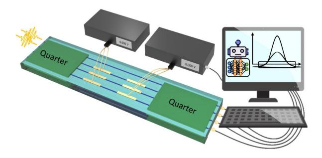
Machine learning for adaptive multiphase estimation with an integrated photonic quantum sensor. Credit: Cimini et al., doi 10.1117/1.AP.5.1.016005.
