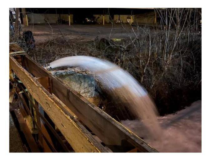
Air-stripping devices, like this one used after the derailment, can help separate chemicals from water. Credit: U.S. EPA
