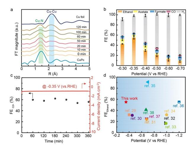
(a) Operando Cu K edge EXAFS spectra for ER-Cu/CuNC under different electrochemical reduction time at -0.30 V; (b) Potential-dependent FEs for different products, (c) Long-term durability at -0.35 V; (d) Performance comparison. Credit: Science China Press
