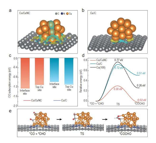
(a-b) Charge density difference map, (c) CO adsorption energy, (d) C-C coupling barriers, and (e) C-C coupling process on different interface sites.
