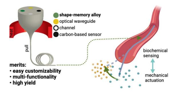
An active fiber fabricated by the thermal drawing. Credit: Sato et al
