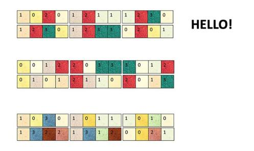
The top row represents the message "Hello!" in quaternary code, which is revealed when the silver nanostructures are illuminated with the correct polarization. The bottom two rows display incorrect sequences when incorrect polarization keys are used. Credit: NAM EPFL
