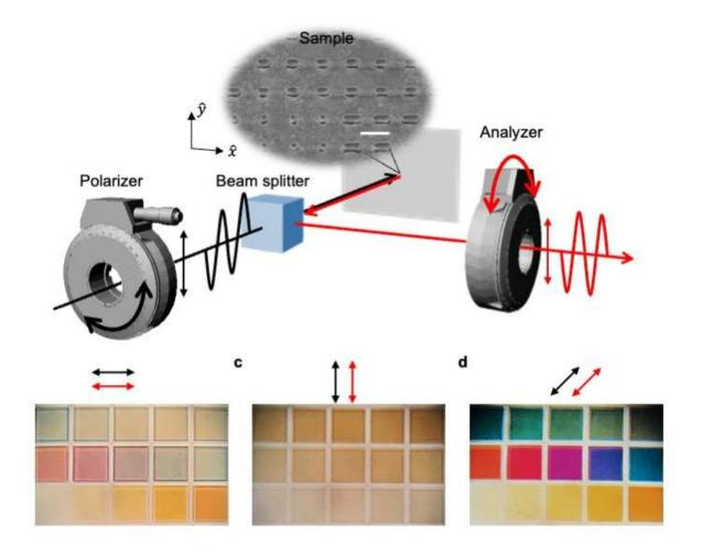
Schematic illustrating the effect of different polarization directions on the colors reflected by the silver nanostructures. Credit: NAM EPFL
