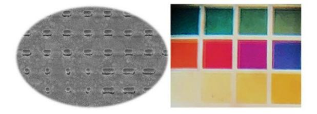
Codable colors (R) reflected by the silver nanostuctures (L) developed in the Nanophotonics and Metrology Lab. Credit: NAM EPFL
