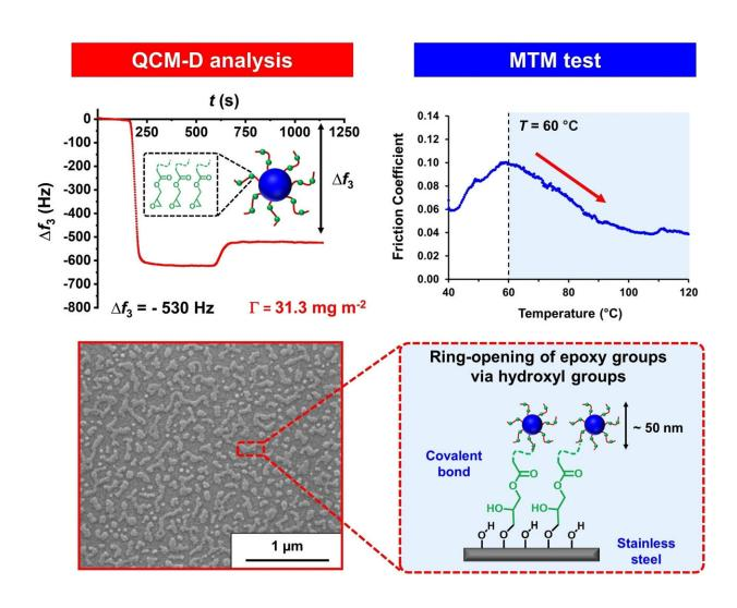
Graphical Abstract. Introduction of epoxy groups into sterically-stabilized diblock copolymer nanoparticles leads to their efficient chemical adsorption onto stainless steel whereas the corresponding non-functional nanoparticles merely
