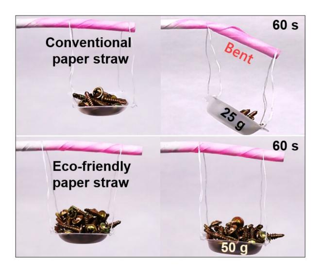
When used to stir a beverage in a cup, a paper straw is frequently bent slightly or delaminated. Due to its high mechanical rigidity in water, eco-friendly paper straw was observed to withstand a relatively heavy weight for 60 seconds under
