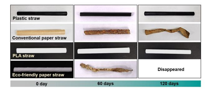
Conventional plastic straws and corn plastic straws did not decompose after 120 days under marine conditions. They have preserved their shape and lost only 5% of their total weight. In the meantime, eco-friendly straws developed by the research team lost more than 50% of their weight after 60 days and decomposed completely after 120 days. Credit: Korea Research Institute of Chemical Technology (KRICT)
