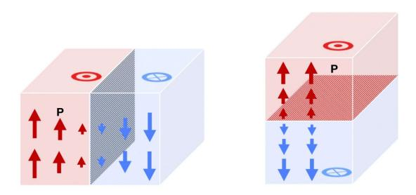
Renderings of a neutral domain wall perpendicular to the surface of a ferroelectric material (left) and a charged wall parallel to the surface (right). Red arrows represent positive charges, with blue signifying the negative. Credit: *Nature* (2023). DOI: 10.1038/s41586-022-05503-5
