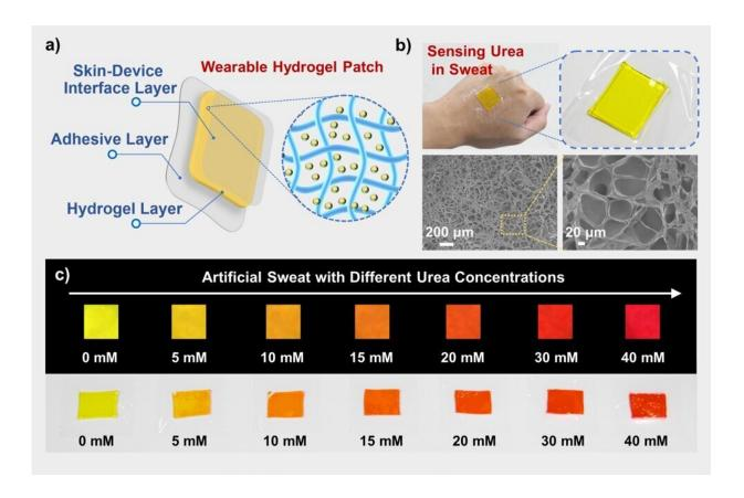
Designed wearable hydrogel sensing patch and response of hydrogel sensing patch to urea under 980 nm excitation and daylight. Credit: Kang Xiaohui
