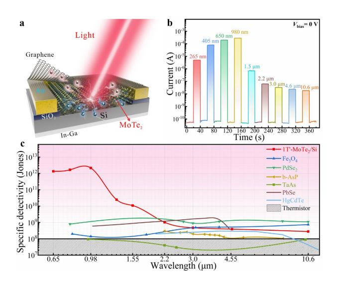
a, Schematic illustration of a graphene/1T'-MoTe<sub>2</sub>/Si Schottky junction device. b,Time-dependent photoresponse properties to pulsed light illumination in a
