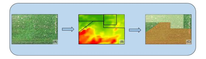
Schematic representation of (A) an aerial image using an unmanned aerial vehicle (UAV) to scout fields in year 1, (B) detection of areas of high (orange) and low (yellow) weed density in year 1, and (C) implementation of year 1 weed maps to calibrate precision planter to plant in high (red) and low (green) crop densities in year 2. Credit: *Weed Science* (2022). DOI: 10.1017/wsc.2022.62
