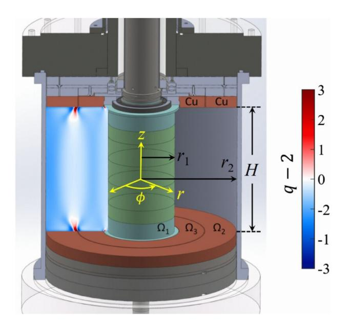
Sketch of the Taylor-Couette cell used in the experiment. The cell has three
