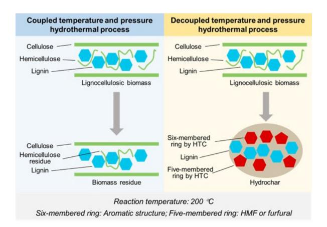
The performance of decoupled temperature and pressure hydrothermal process. Credit: the authors
