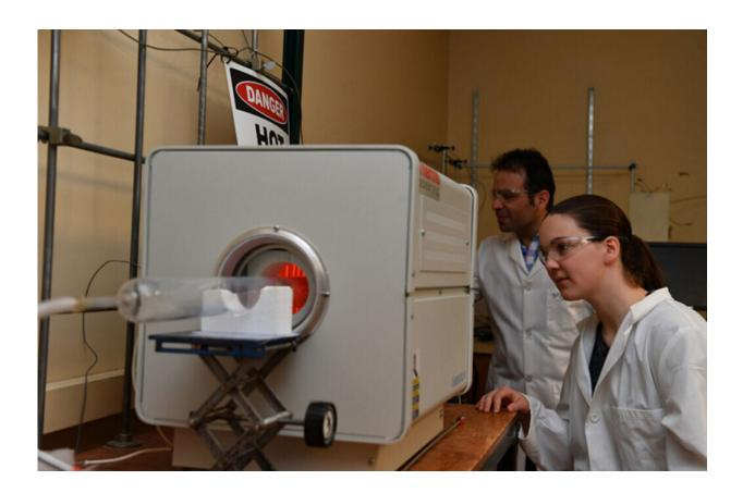
Chemical Engineering PhD Candidate Wrya Aframehr and undergraduate student Constance Kirby work with a high temperature reactor to produce ammonia via chemical looping of manganese. Credit: Washington State University
