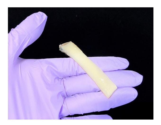
The new squid/synthetic polymer double-network gel developed in this study. Credit: Tasuku Nakajima
