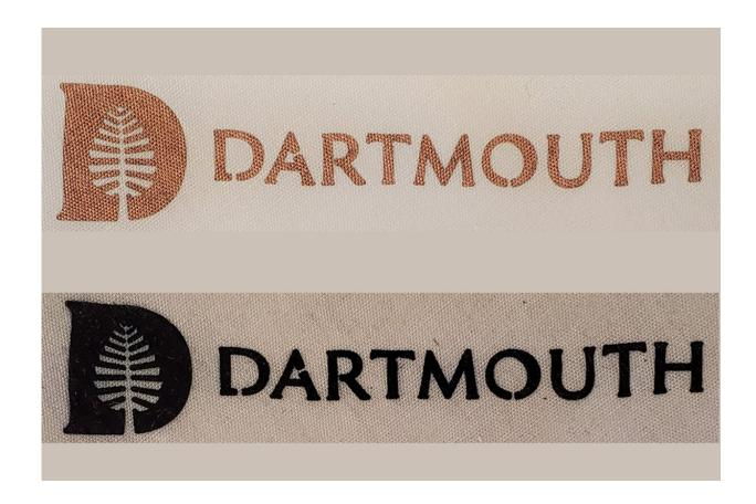
Copper imprinted on fabric (top) is replaced with a metal-organic framework (bottom) capable of detecting and capturing toxic gases. Credit: Katherine Mirica
