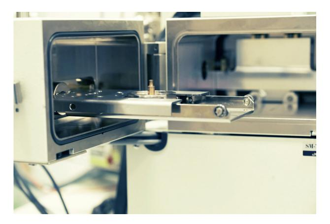
A sample in a scanning electron microscope used in Nanyang Technological University, Singapore's quantum recoil experiments. Credit: NTU Singapore
