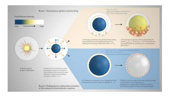
The flame front at its formation (a and b) and during normal knock (c and d) or super-knock (e and f). The Route 1 mechanism favors knock, while the Route 2 mechanism leads to super-knock. Credit: Sandia National Laboratories
