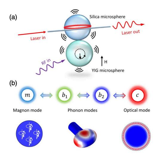
Schematic of the hybrid system that combines controlled phonons, magnons, and photons. Credit: Shen Zhen et al
