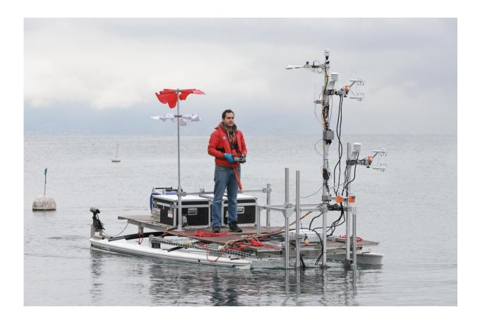
Mehrshad Foroughan used an array of measuring instruments including an unmanned, GPS-guided catamaran. Credit: Alain Herzog
