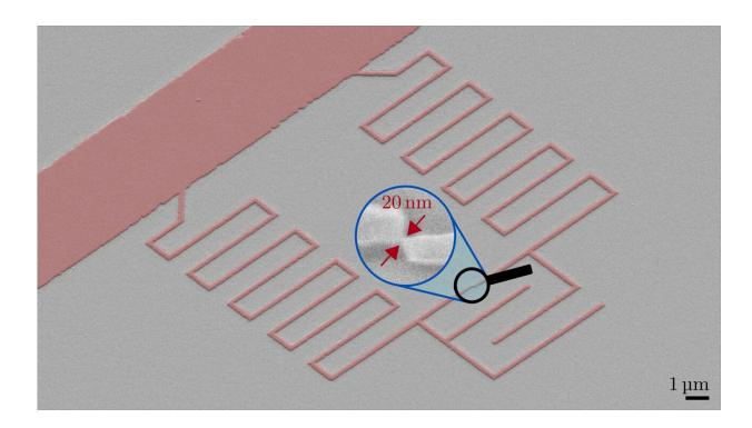
The properties of gralmonium qubits are determined by a small junction of 20 nanometers only, which acts like a magnifying glass for microscopic material defects. Credit: Dennis Rieger, KIT
