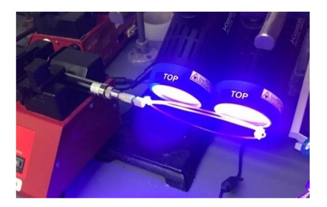
A mild solution containing reagents passes through an illuminated loop in a Rice University laboratory. The lab has developed a photochemical process to simplify the synthesis of drug and chemical precursors known as diamines. Credit: West Research Lab/Rice University
