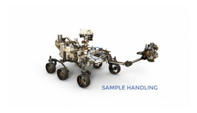
The Perseverance rover's sample handling equipment is located in the blue circle on this image. Credit: NASA/JPL-Caltech/MSSS
