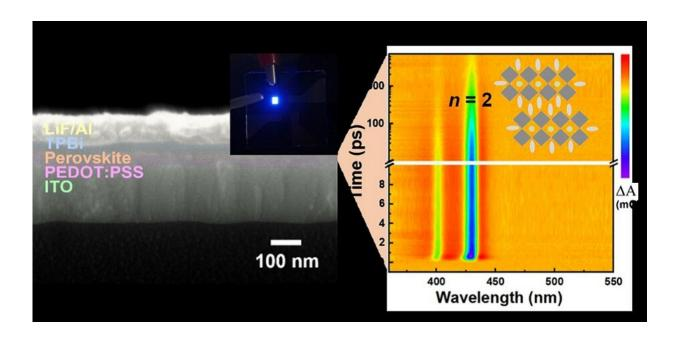
Scanning electron microscopy image with digital photograph during operation (left) and transient absorption spectrum (right) of deep-blue emitting perovskite light-emitting diodes (LEDs) prepared by hot-antisolvent bathing. Credit: J. Moon, Yonsei University.
